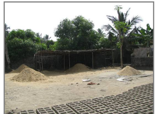
Cinder blocks molded on campus premises
